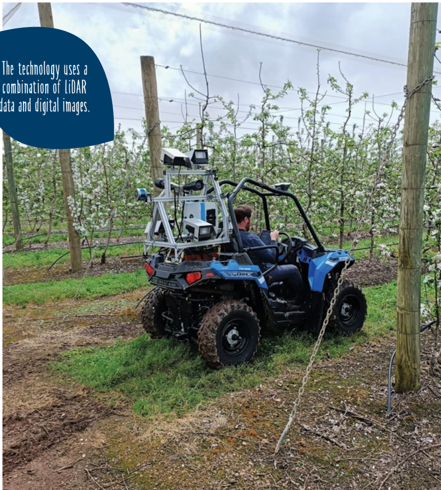
► CARTOGRAPHER collecting digital images at bloom in an 'ANABP 01 01 ' block at Newton Orchards, Manjimup.
